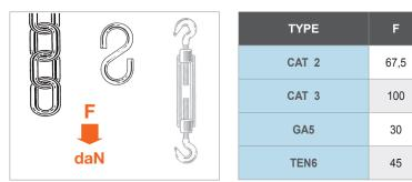
Recommended load is the average resistance loads with a safety coefficient. 1daN=1kg.
