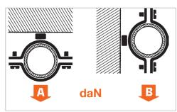
Tests were carried out in technical laboratory with a dynamo-metric machine. For wall fixing, stick to the strength characteristics of the plug or the connecting support.
