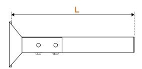
A PAPS, and N° 2 JBR10 with a tightening torque of 40 Nm have been used for PF3 strut channels.
