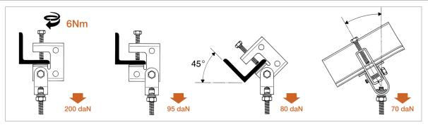
Recommended load is the average resistance load with a safety coefficient. Tightening torque = 6 Nm. 1 daN=1 kg
