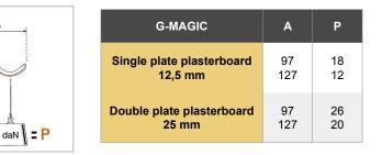
Recommended loads refer to the single bracket, also considering the related base material. Load capacity is highly influenced by the plasterboard plate's density. 1daN=1 kg.
