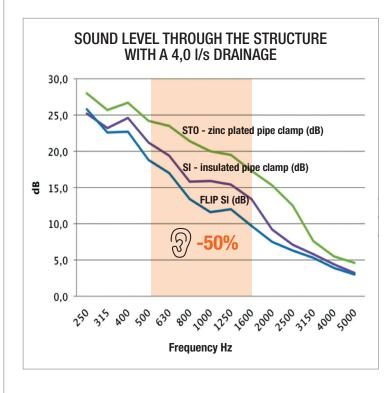
Laboratory test provided by Istituto Giordano (Gatteo ,FC, Italy) to measure the amount of noise produced by waste water systems according to the UNI EN 14366:2005 regulation.
