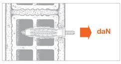
Recommended load is the average resistance loads with a safety coefficient. Data expressed in daN. 1daN = 1 kg.
