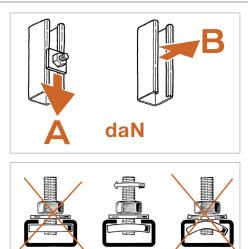
Recommended load is the average resistance loads with a safety coefficient. 1 daN=1 kg.
