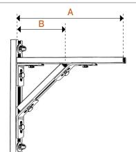
Static loads Material: DX 51 D - D D11
